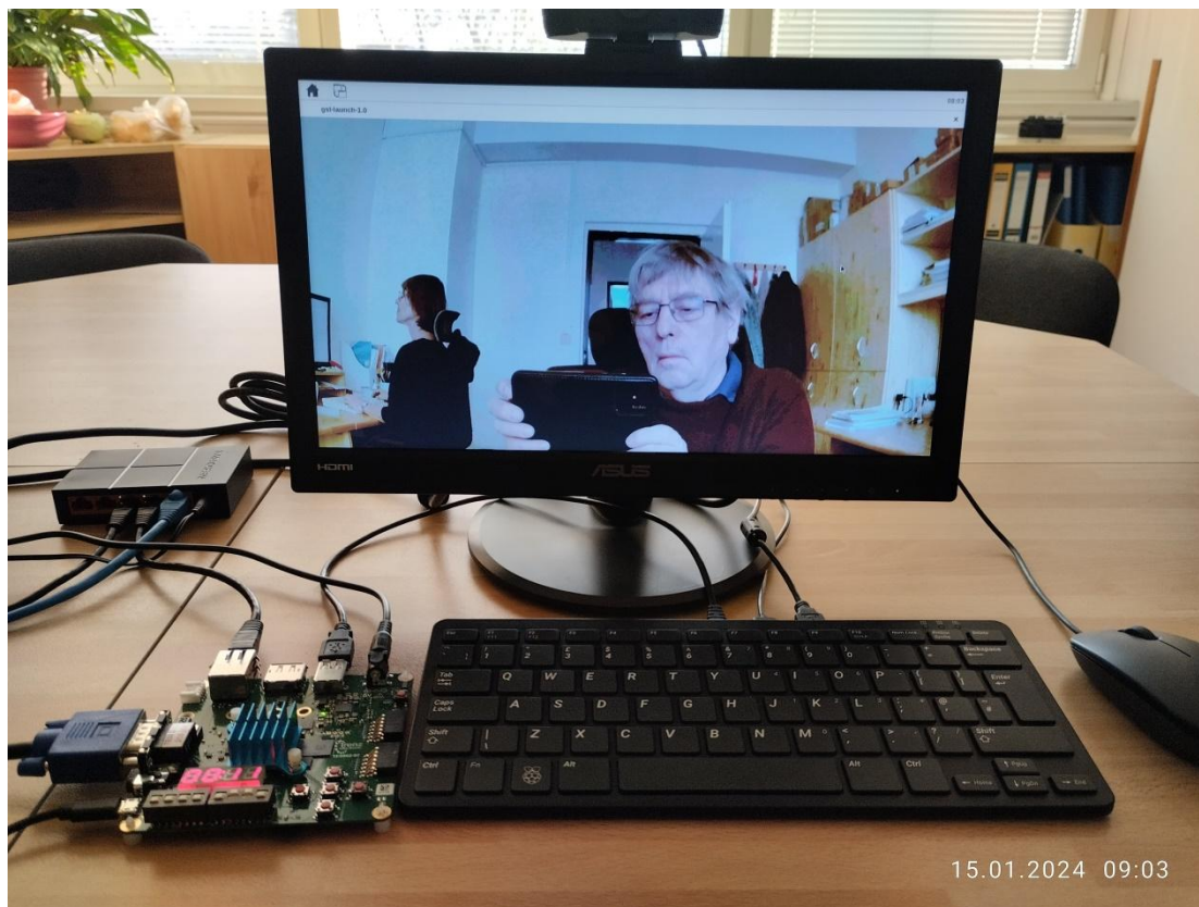
Full HD video from USB camera is converted to local HD VGA RGB444 display.
