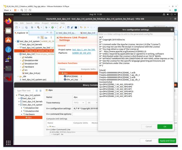
Click "..." button on the line of V++ Configuration Settings and modify configuration as follows:
