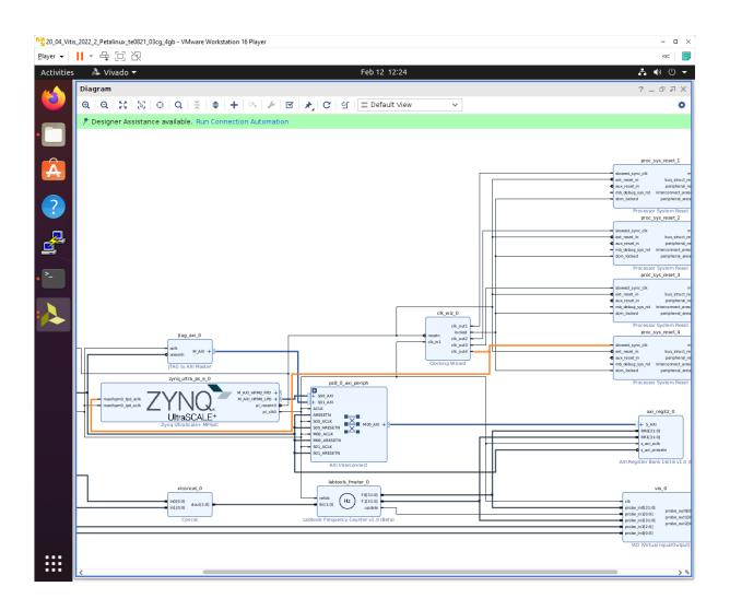
Double-click on **zynq\_ultra\_ps\_e\_0** block and enable **M\_AXI\_HPM0\_FPD** port. Select data width 32bit. It will be used for integration of inerrupt controller on new dedicated AXI stream subsystem with 240 MHz clock. It will also enable new input
