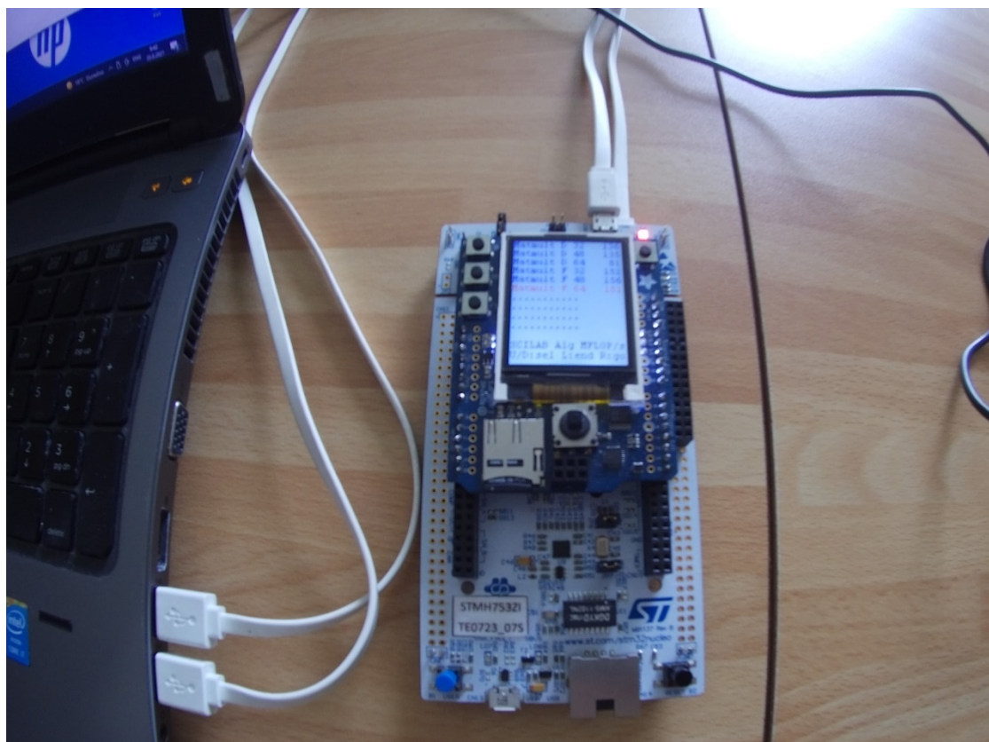
Figure 15: STM32H753 terminal screen defined by scilab-cli script top_mult3.sce
