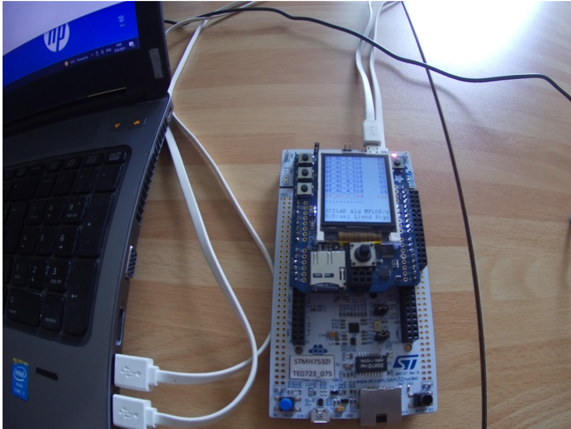
Figure 16: STM32H753 terminal screen defined by scilab-cli script top_md51d.sce
