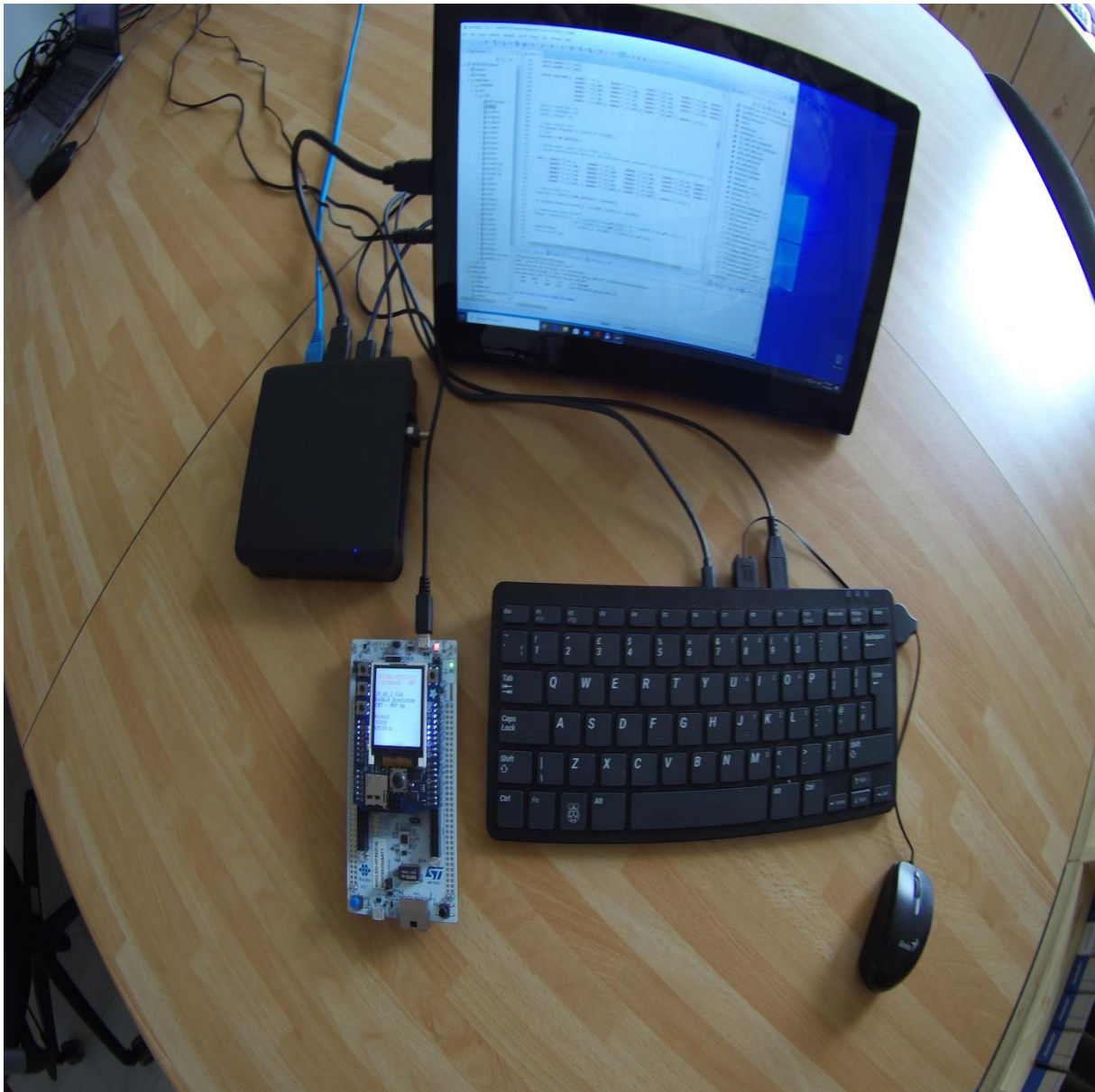
Figure 38: Double precision system identification, STM32H755ZI-Q board, CM7 MCU
