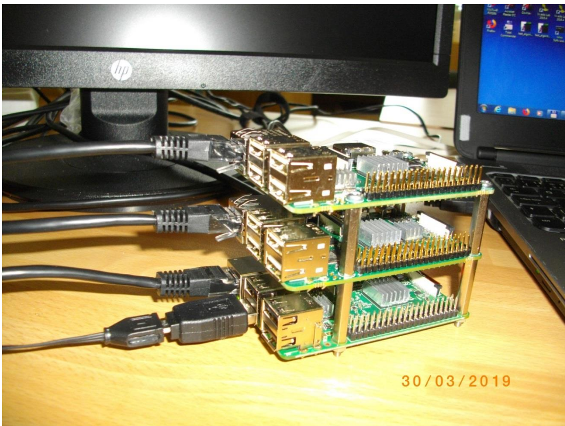
Figure presents: RPi3 (bottom), and two ZynqBerry boards with the Arrowhead framework G4.0 compatible C++ clients running on ZynqBerry boards.
