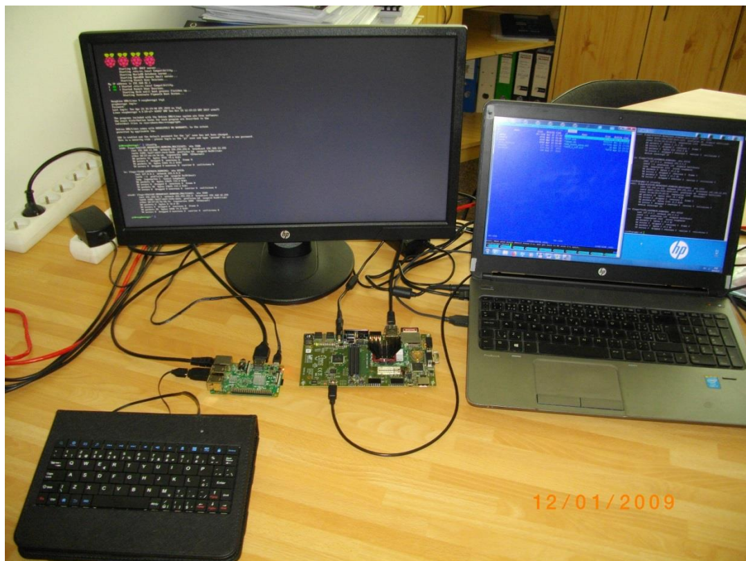
Figure 5: The Zynq Ultrascale+ system and RaspberryPi 3B with Arrowhead framework
