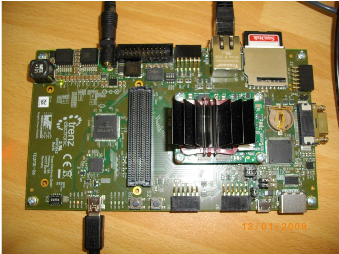
Figure 4: Zynq Ultrascale+ module on TE0701-06 carrier board
