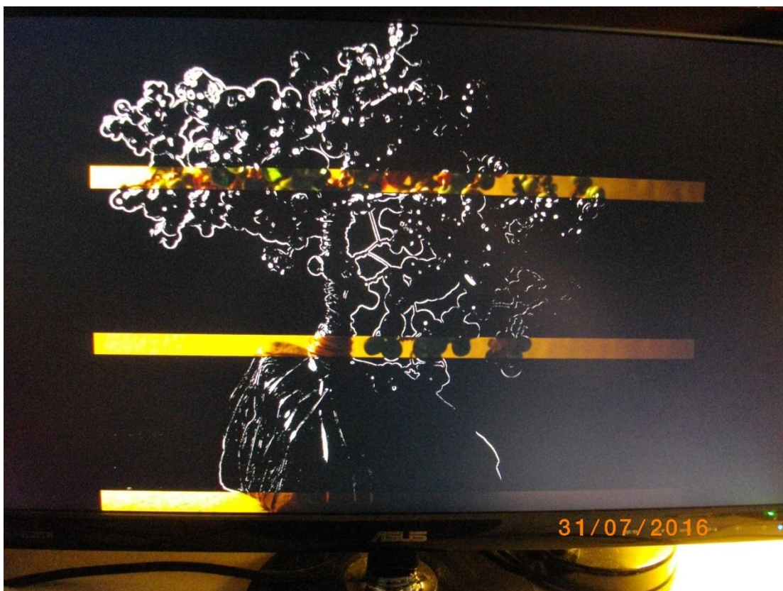
Figure 25: Edge detection (sh03 - Sobel filters, 3 variable HW paths) output on HDMI monitor.
