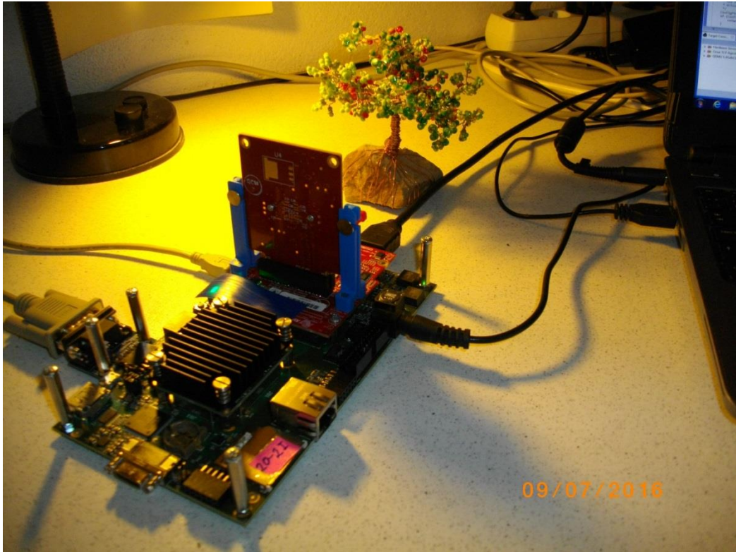
Figure 32: Accelerated edge detection Toshiba sensor and Zynq with EdkDSP.
