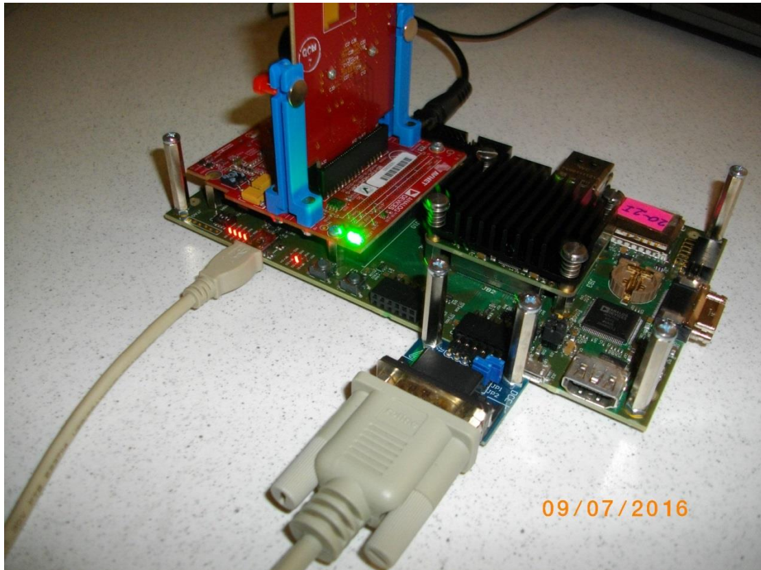
Figure 22: Serial cables USB based for Arm and Jtag. RS232with Pmod for Microblaze .
