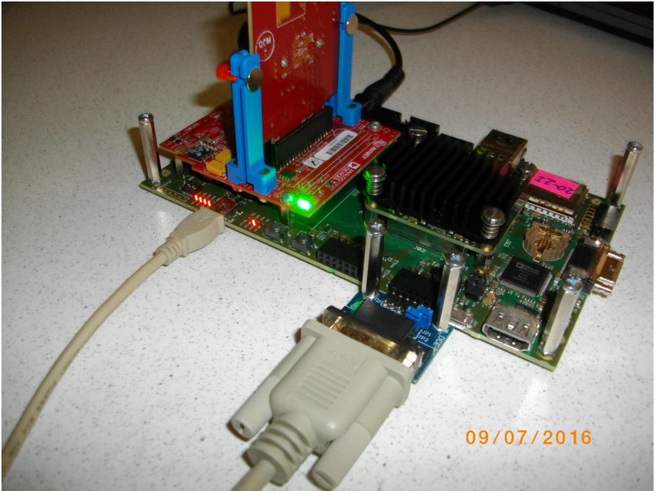
Figure 18: USB for ARM terminal and JTAG. RS232C Pmod for MicroBlaze.
