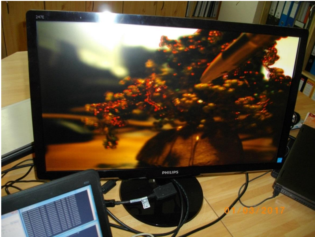
Figure 44: HW accelerated motion detection algorithm – moving edges marked by red.
