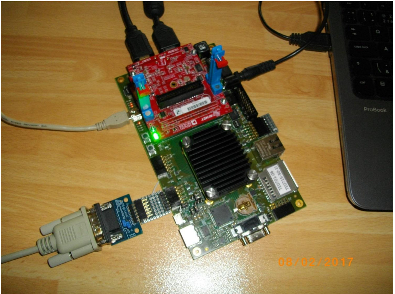
Figure 25: USB for ARM terminal and JTAG. RS232C Pmod for MicroBlaze
