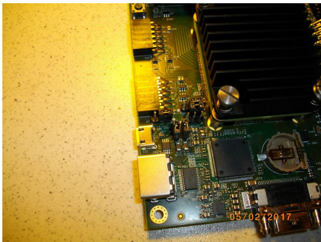
Figure 15: TE701-06 setting of switch S3: 1=OFF 2=OFF 3=ON 4=OFF
