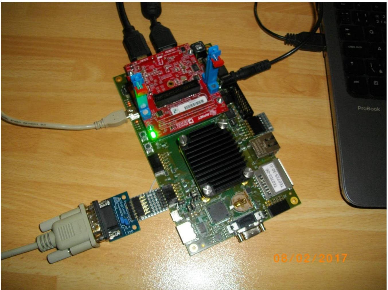
Figure 1: TE0701-06 carrier TE0715-04-30-3E running HDMII-HDMIO in HW and 3x EdkDSP accelerators.
