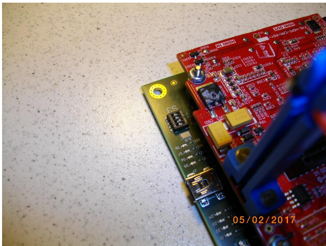
Figure 15: TE701-06 setting of switch S3: 1=OFF 2=OFF 3=ON 4=OFF
