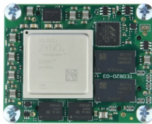
Figure 9: TE0820-3EG SoM [2], the figure shows a similar product.
