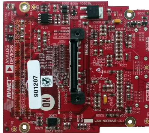
Figure 10: Avnet HDMI Input/Output FMC Module [3].
